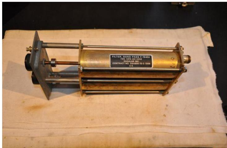
**Twin cavity Filter F-194 / U.** 142-163MHz
