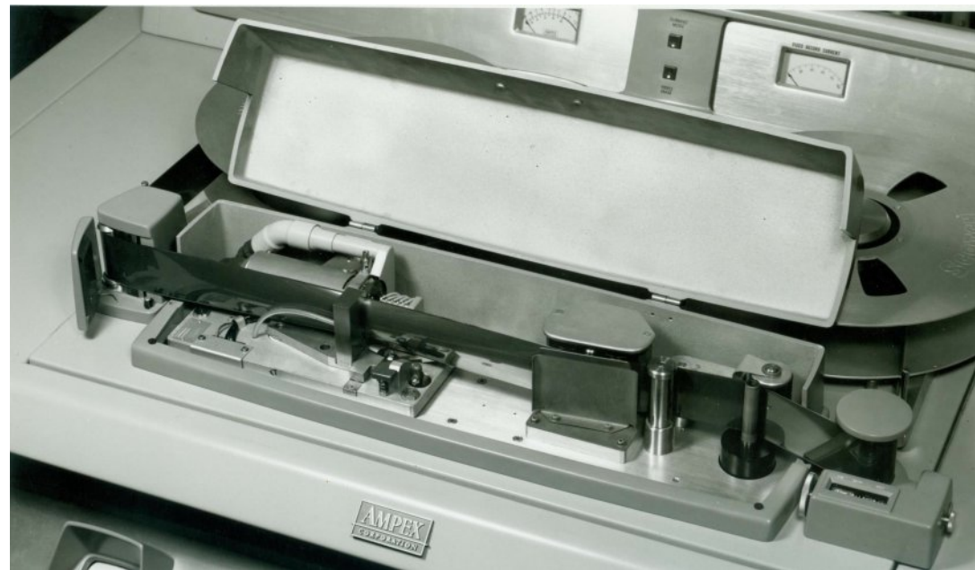
Fig. 25 - VR1000 Top plate with video head assembly and audio, control track heads, and full track erase head assembly
